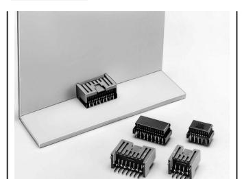
Self-supporting style board to board connectors. Both plugs and receptacles are supplied radial-tape mounted (conforming to JIS C 0805 tape specification), which can be mounted by versatile, radial component pick and place machines. Automatic mounting is possible up to 15 circuits.
